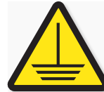
Electric Ground Hazard
