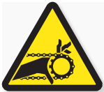
Chain Drive Entanglement Hazard
