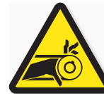
Belt Drive Entanglement Hazard
